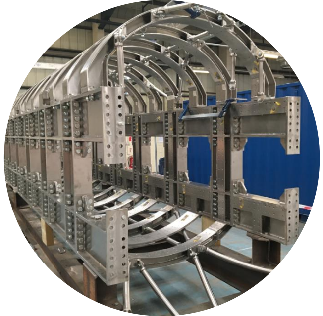
Stainless steel support structure to be installed in the sewer.
